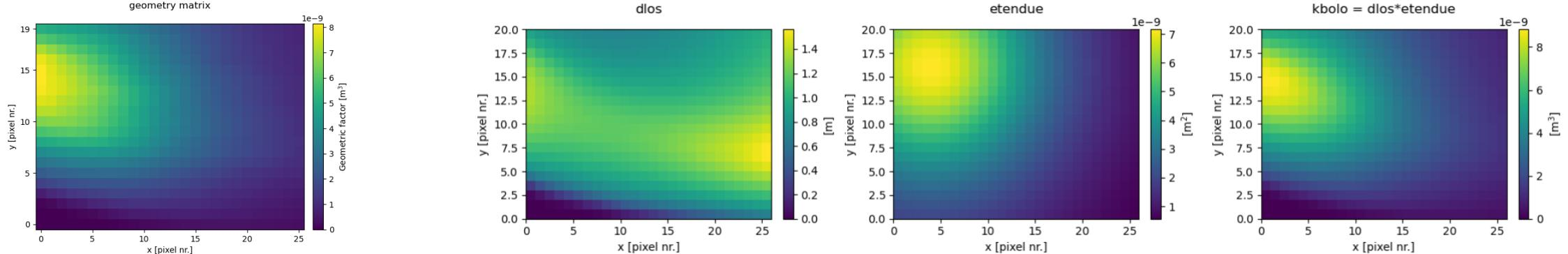
The raw power load data is usually divided by the so-called  $k_{bolo}$  factor, defined as the product of the two, to disentangle the plasma emissivity features from the specific camera geometry. This normalized quantity is named **chord brightness**  $P_{chord}$ .
