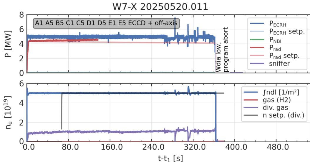
6 min plasma (363s) with  $P=4.9$  MW → **new injected energy record of 1.785 GJ**
