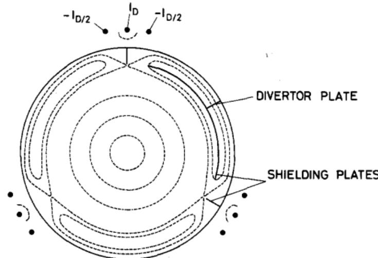
Fig. 5. Cross section of a helical divertor with triplet helical windings outside the vacuum chamber and shielding plates only in the outer section of the torus (resonance at  $q = 3$ ,  $I_D/I_p = 0.08$ ).
