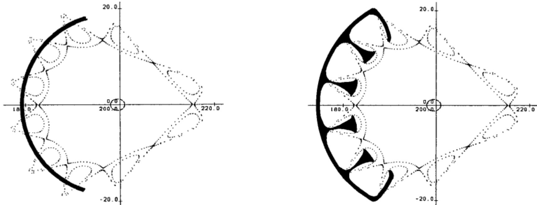
Fig. 1: First proposal of an open (left) and “closed” (right) ID geometry, applied to a W7-AS island configuration.
