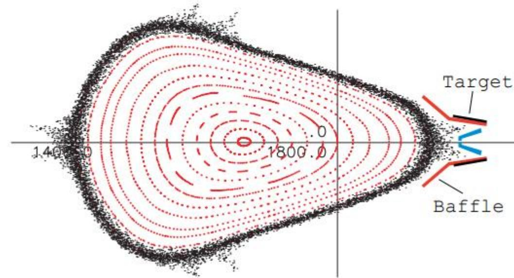
**Figure 5.** Poincaré plot of magnetic surfaces and the scrape-off layer in the symmetry plane  $\varphi = 45^\circ$ . The stochastic region is created by the intersection points of diffusing particles.
