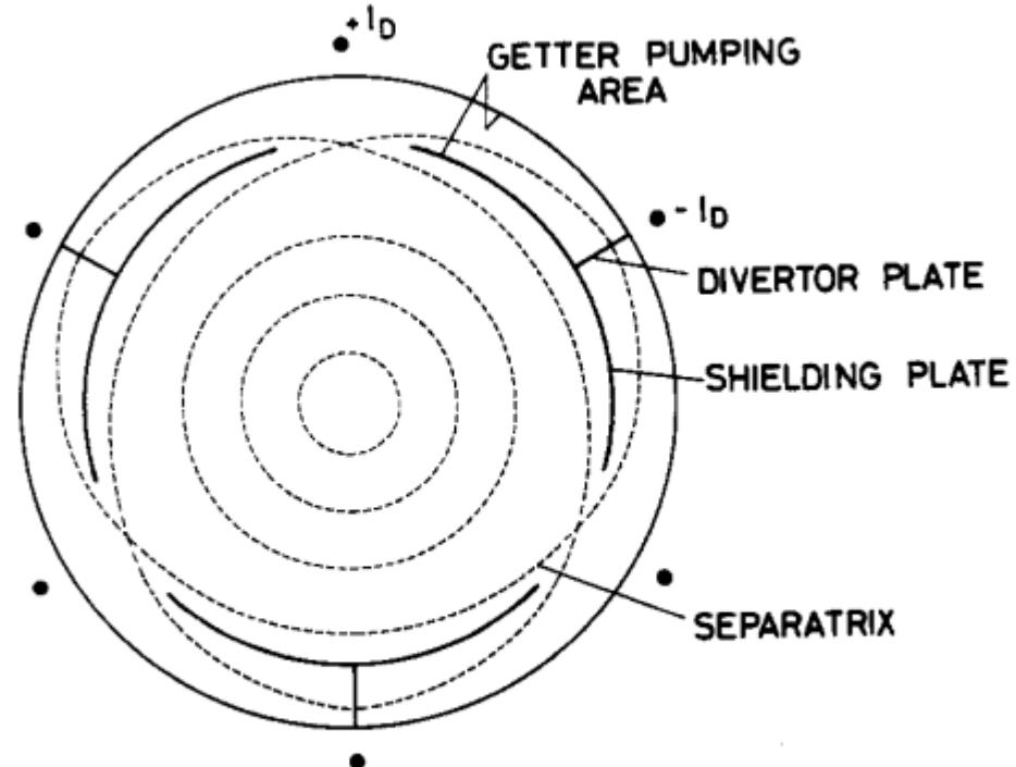
Fig. 1. Schematic picture of the cross-section of a helical divertor with resonance at  $q = 3$  ( $I_D/I_p = 0.01$ ).
